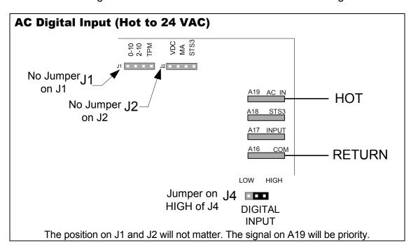
Connect the control signal wires to terminals A16 and A19 for an AC signal.
